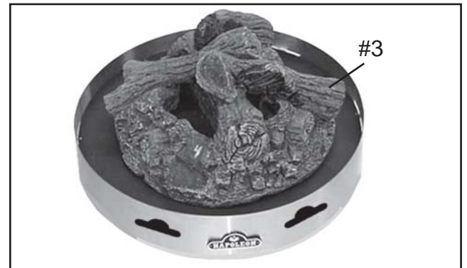
4.1.4 Hook log #3 into notch on base log.
